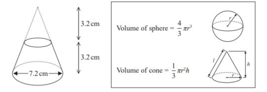
The diagram shows that the frustum is made by removing a cone with height 3.2 cm from a solid cone with height 6.4 cm and base diameter 7.2 cm.
